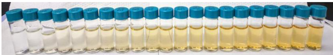
Figure B-1. Calibration series for ammonia colorimetry by Nessler method.
