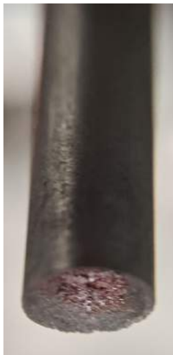
Figure 2-16. A hollowed graphite working electrode, with the produced cavity smeared with red phosphorus for nonfaradaic in situ P 4 generation.
