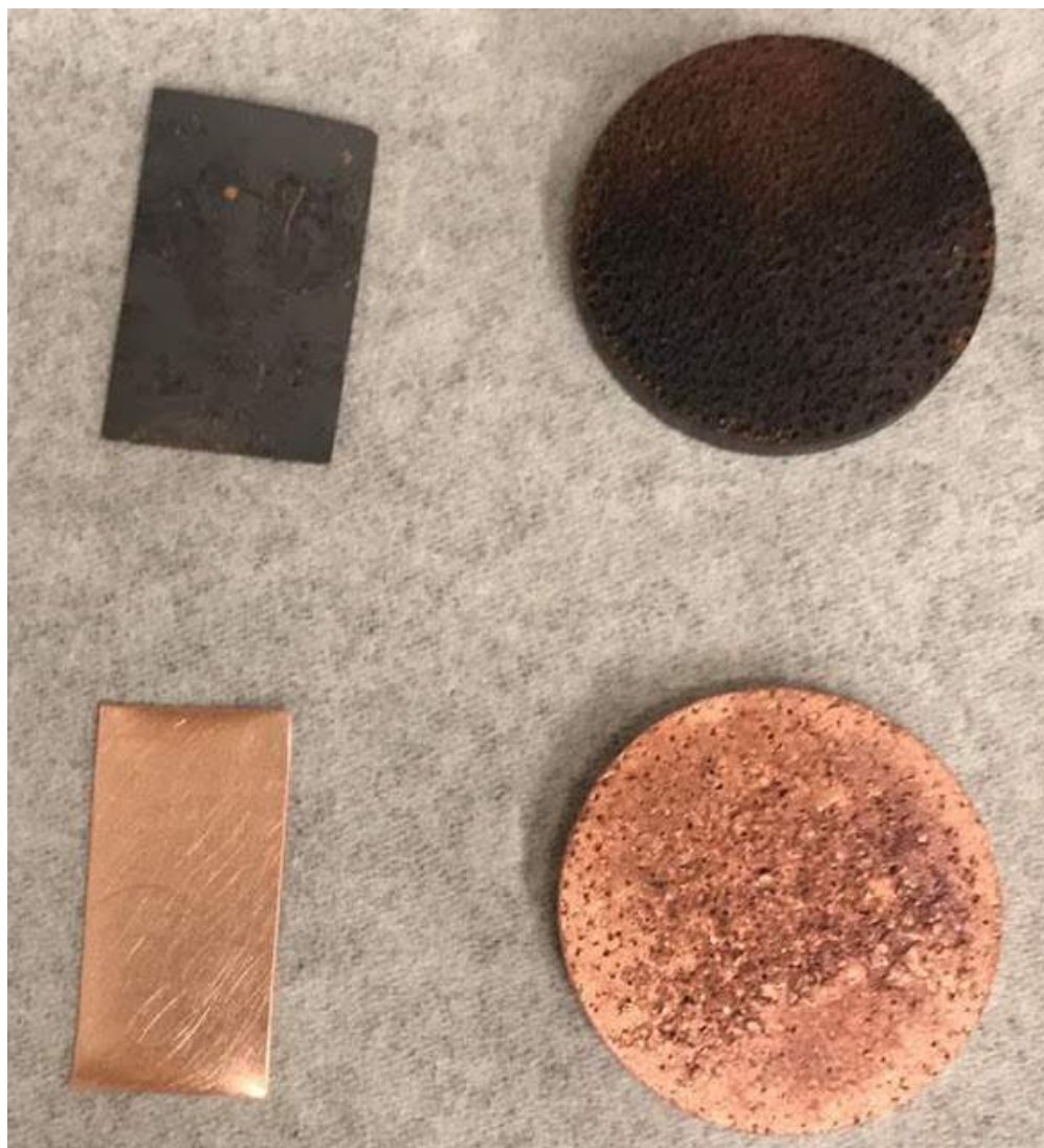
Figure 3-21. (top) Copper foil and foam nitridated by sodium amide prep. (bottom) Copper foil and foam nitridated by flowing-ammonia prep.
